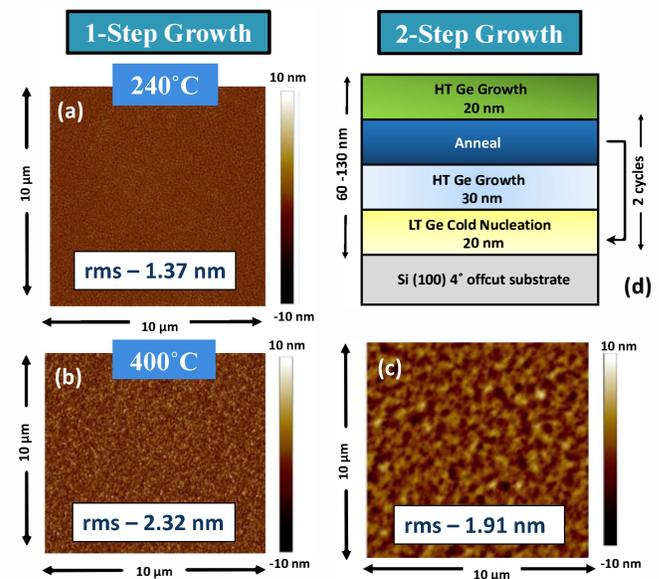
**Fig. 4** AFM micrographs for (a) sample A, (b) sample B, and (c) sample C and (d) the growth sequence of sample C.
