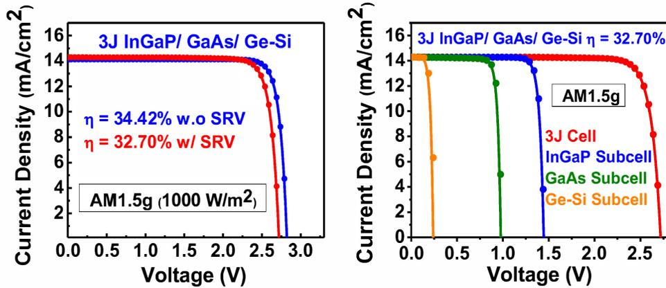
**Fig. 3** Current-matched JV characteristic of 3J InGaP/GaAs/Ge-Si solar cells (a) with and without taking into account SRVs, (b) Current-matched JV characteristics for 3J InGaP/GaAs/Ge-Si and individual subcell stacking into account SRV under AM1.5g, 1-sun.
